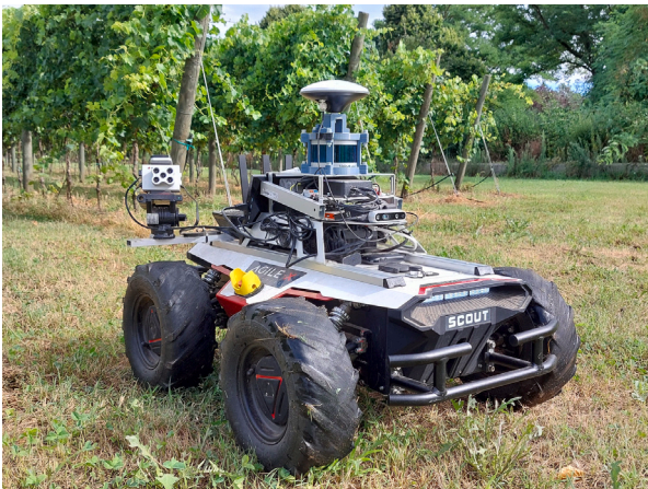
Fig. 1. The mobile robot in vineyard used to collect the FriülBot dataset.
