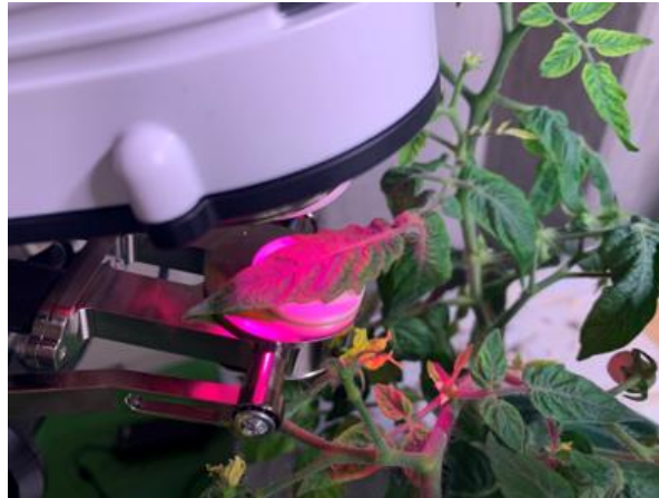
Figure 3. Infrared Gas Analyzer (IRGA) with a fluorometer leaf chamber used to simultaneously measure gas exchange and chlorophyll fluorescence.
