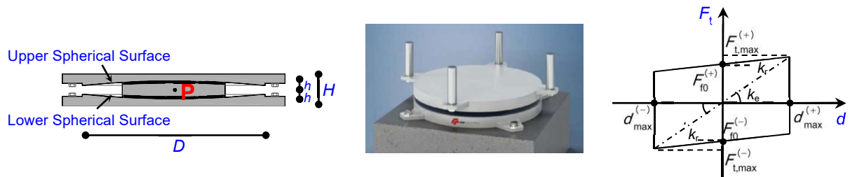
Fig. 9 Cross section, view and schematic response cycle of a DCSS isolator with equal sliding surfaces
