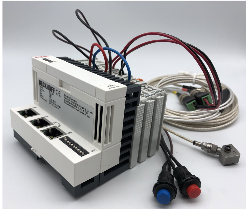
Figure 2.10: Edge device configured for the demonstrative system
