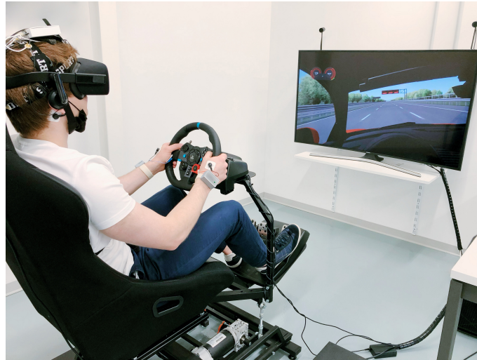
Figure 6. A test subject in our lab using our simulator setup, with SPR, ECG, and EEG sensors employed to acquire the physiological signals (Experiment 2).
