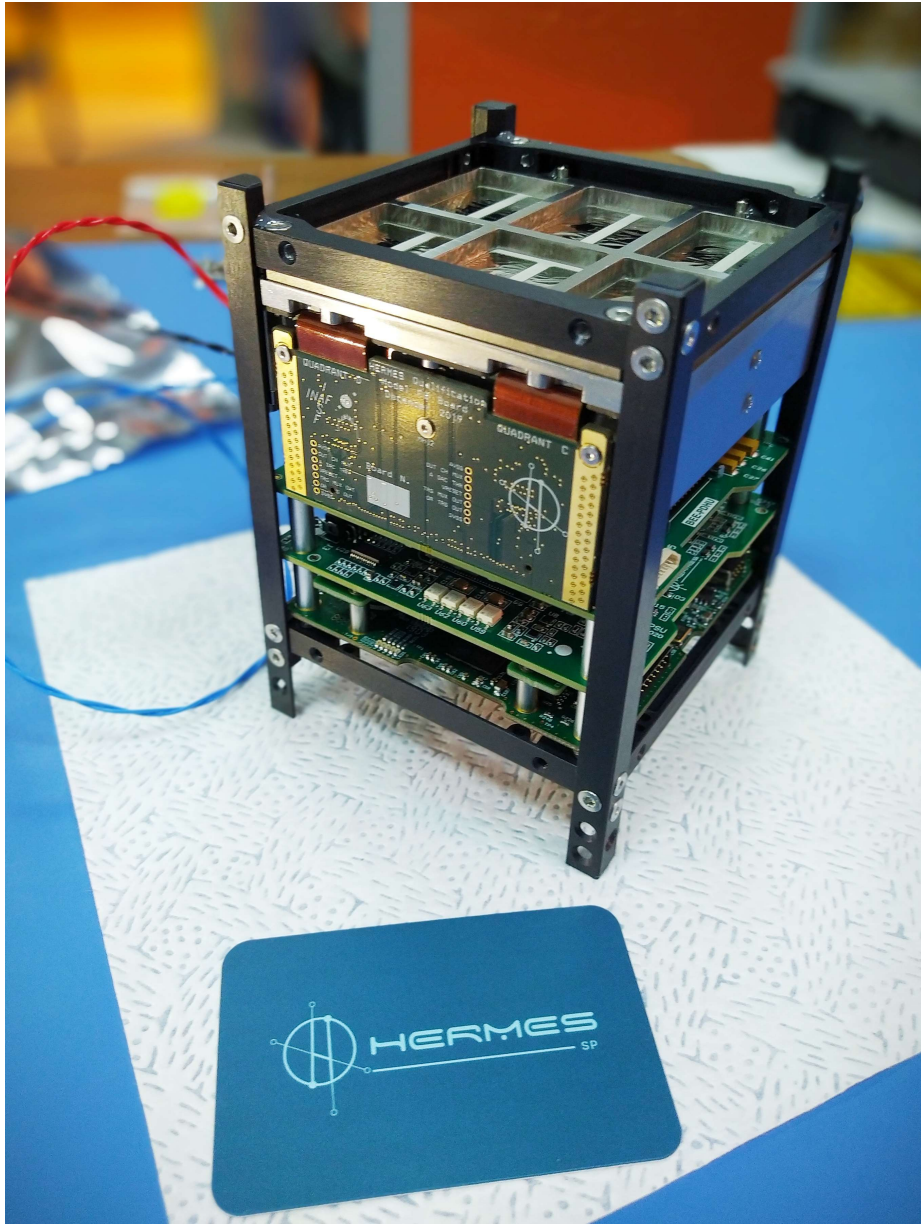
Figure 2.3: The HERMES payload demonstration model. From top to bottom the detector assembly, the BEE board and the PDHU's main and daughter boards are distinguishable.
