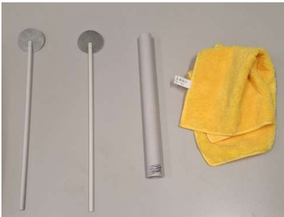
Figure 9.7: A pair of metal plates with plastic handles (on the left) used to explore the electric properties of the space surrounding a charged body. For a rough measurement, it may be a PVC tube charged by rubbing it with a microfibre cloth (on the right).
