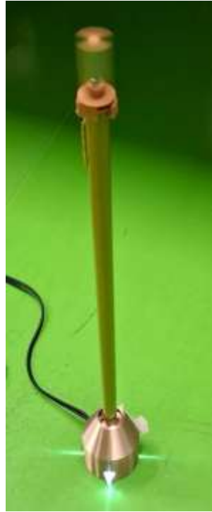
Figure 9.8: Electric field sensor working to verify the vector sum regular and to calculate the circulation along a generic curve.
