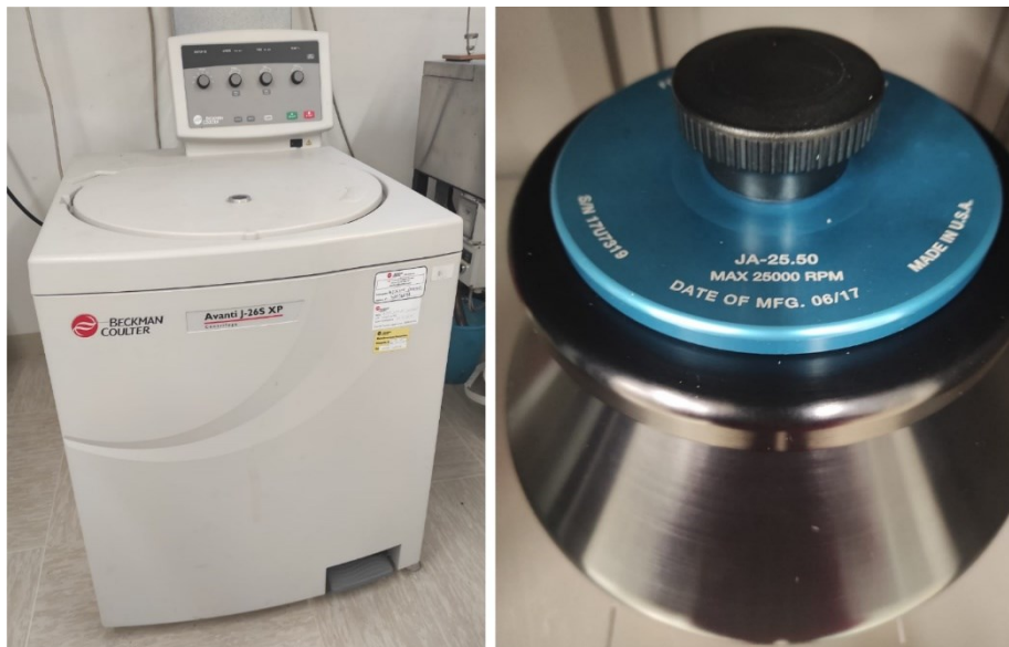
Figura 10: Centrifuga Beckman Coulter Avanti J-26S XP e rotore Beckman Coulter JA-25.50
