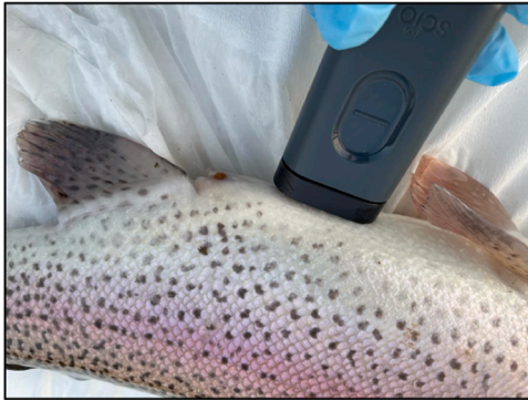
Fig. 2. Adult rainbow trout analysed with the SCiO sensor over the abdominal area.
