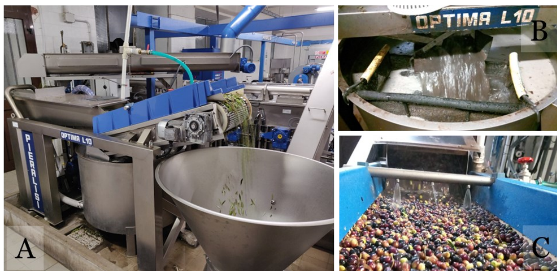
Figure 1.4. Olive washing machine (A) comprising the washing tank (B) and the conveyor belt with water jets for the final rinse (C).
