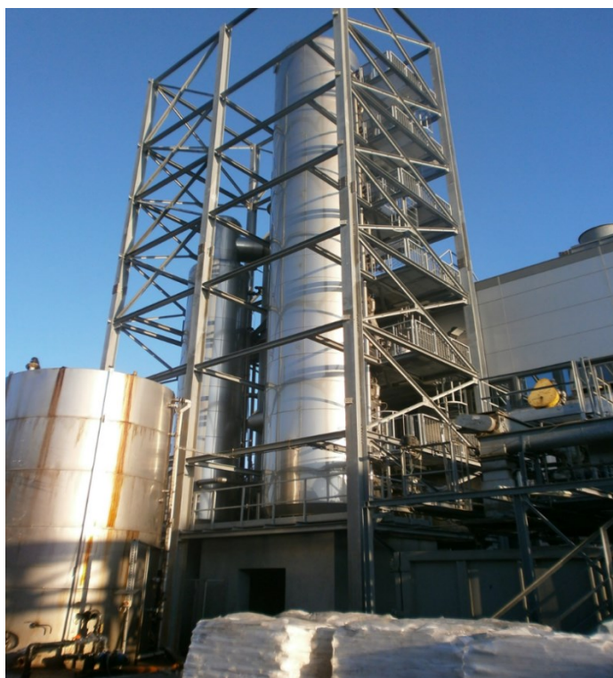
Figure 1.16. Distillation column for oil deodorization.
