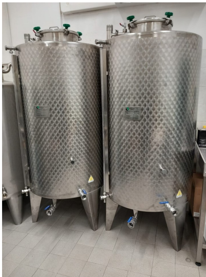
Figure 1.10. Stainless-steel tanks for oil storage.
