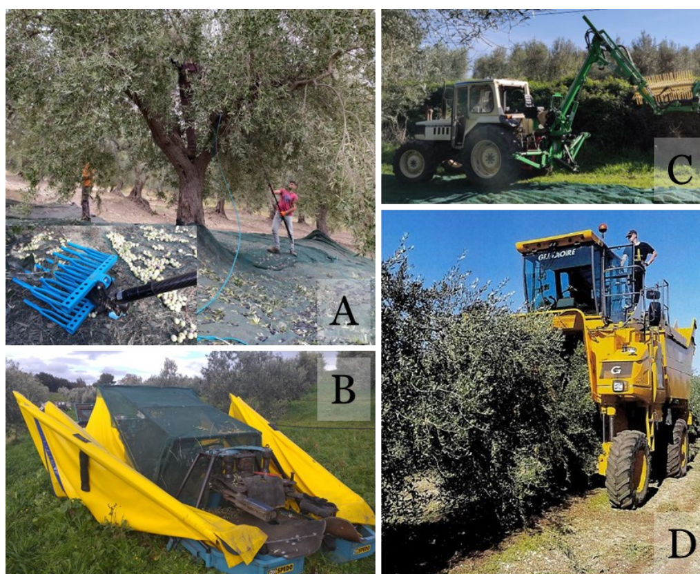
Figure 1.2. Harvesting of the olives carried out with hand-held combs (A), trunk shaker equipped with the collection umbrella (B), vibrating comb mounted on a tractor (C) and straddle harvester (D).
