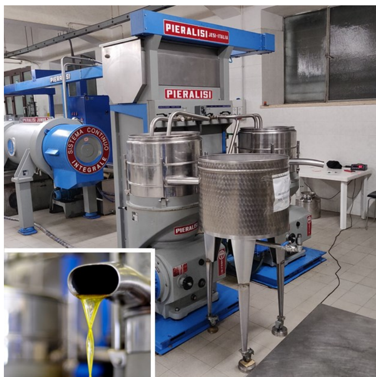
Figure 1.8. Disc centrifuge, with detail of the oil outlet.
