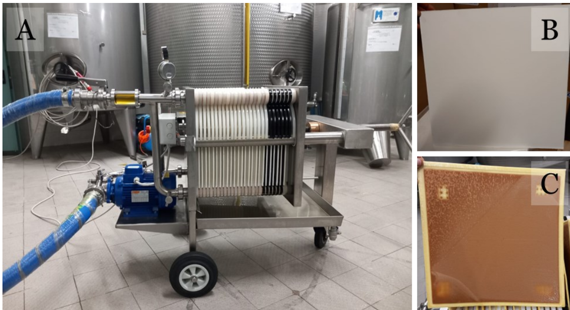
Figure 1.9. Oil filtration system with horizontally stacked filters (A). Filter before (B) and after (C) filtration.
