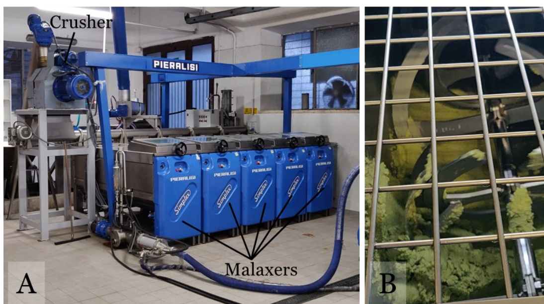
Figure 1.6. Battery of malaxers fed by the crusher (A) and detail of the olive paste under mixing by the rotating blades (B).
