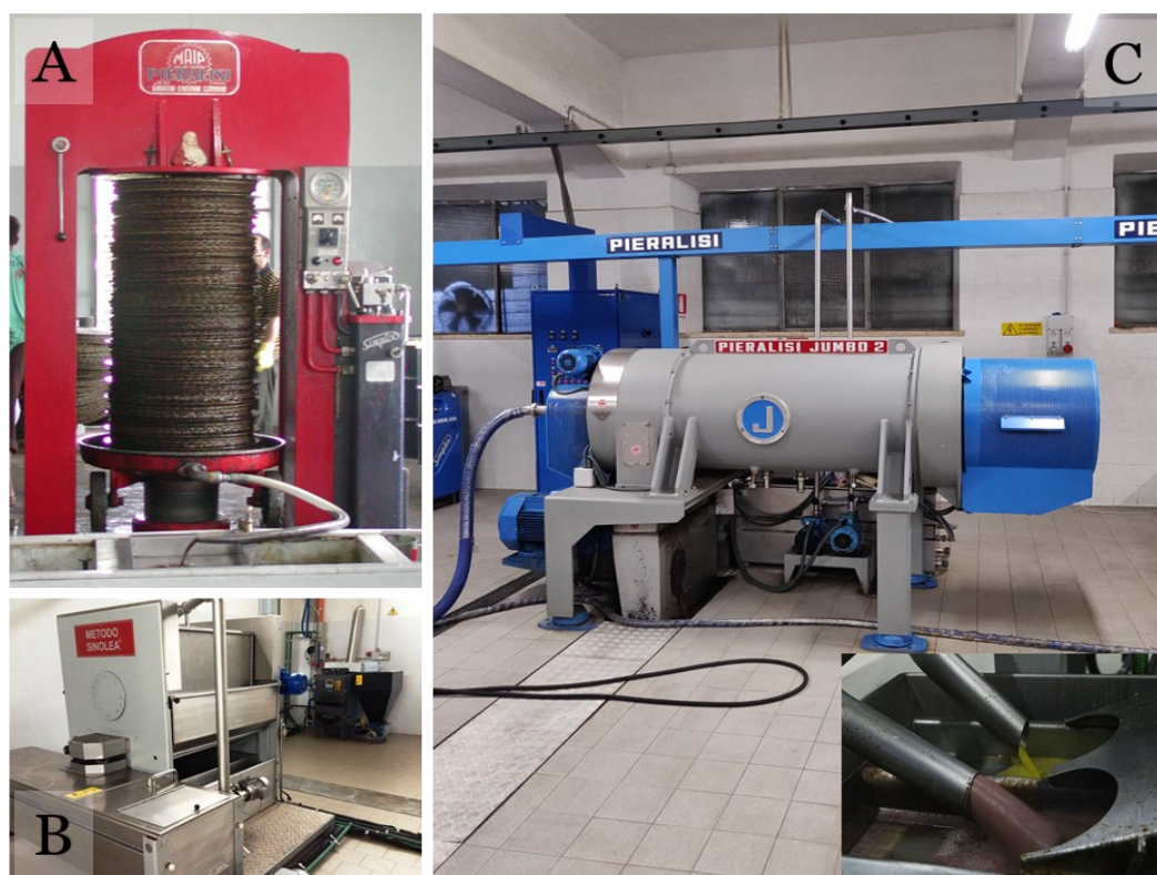
Figure 1.7. Extraction of olive oil from olive paste by pressing (A), by percolation using a Sinolea system (B) and by centrifugation using a three-phase decanter, with detail of vegetation water and oil outlets (C) [adapted from www.oliveoil.com (A) and www.frantoionline.it (B)].
