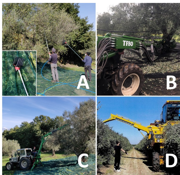
Figure 4.1. Olive harvesting carried out by hand-held comb (A), trunk shaker (B), mechanized vibrating comb (C) and straddle harvester (D).
