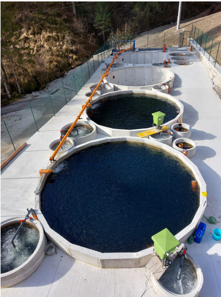
Figure 1: Slovenian rainbow trout recirculating aquaculture system (RAS).
