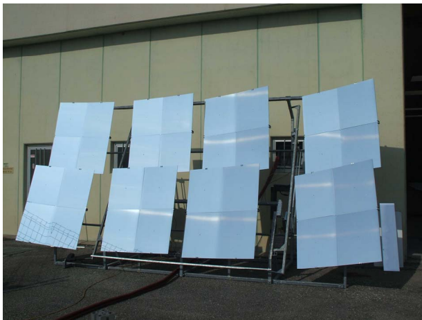
Figure 3. A Linear Mirror II device with eight mirrors.
