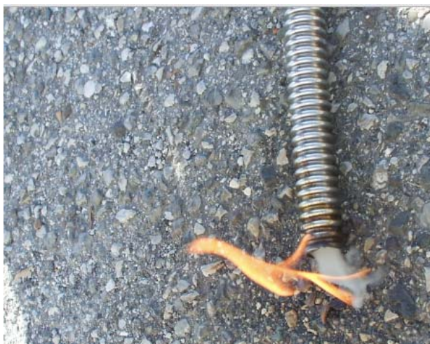
Figure 8. Flame at the exit of the torrefaction steel tube.
