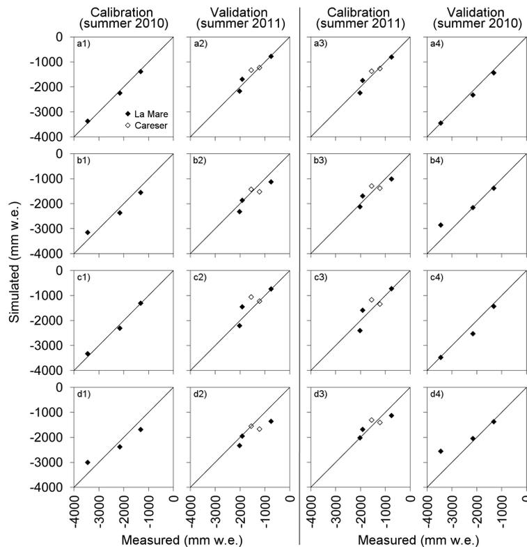
**Figure 10.** Measured vs. modeled mass balance at the eight glacial weather stations, using EISModel with four different air temperature inputs: (a1–a4) measured, (b1–b4) extrapolated from Car\_2607 via the standard lapse rate ( $-6.5^{\circ}\text{C km}^{-1}$ ), (c1–c4) calculated via the G&B method, and (d1–d4) calculated via the S&M method. Corresponding statistics are reported in Table 5.
