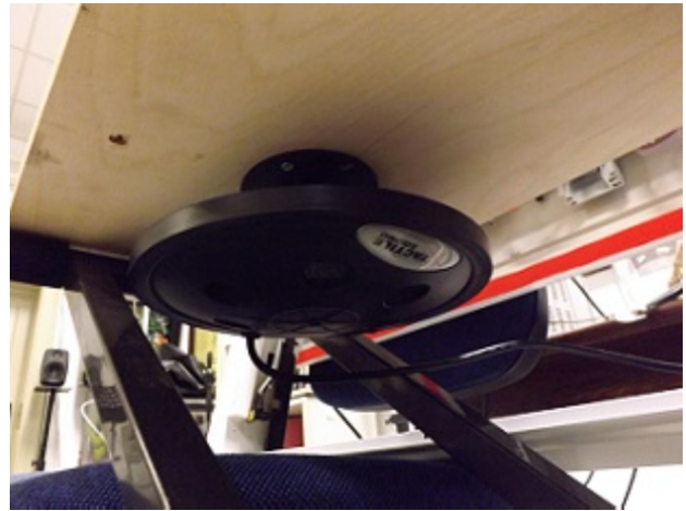
Figure 2. One of the transducers used to convey vibration at the keyboard.
