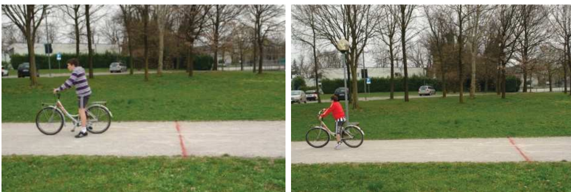
Figure 3. Stopping distances using rear brakes at two different speeds, 15 km/h (left) and 20 km/h (right): activity performed by middle school pupils.
