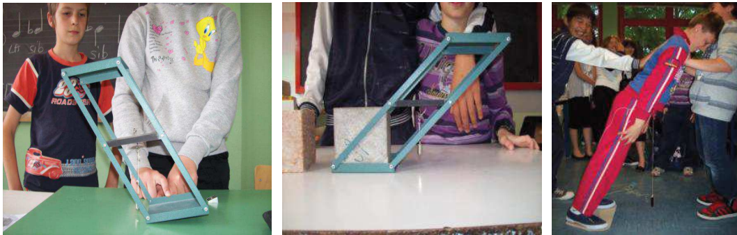
Figure 5. Explorations of the equilibrium conditions with school laboratory objects (left, center) and with pupils (right).
