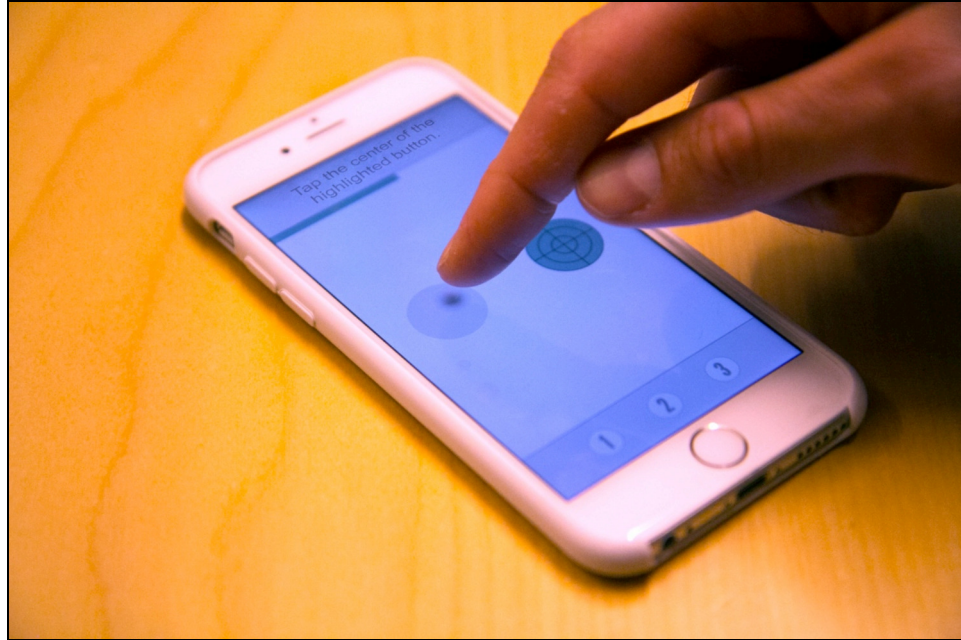
Figure 7: Feedback provided by the TAPPING2 motor test. The black circle on the screen indicates the position on which the user has just tapped. In this picture, the smartphone is kept on the table for demonstrative purposes.
