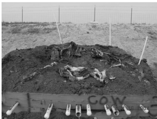
Figure 1. Platforms used to compost adult dairy cows, using dried solids separator manure as a composting amendment. Pipes protruding from wood sides allowed sampling of leachate that could penetrate the soil beneath the carcasses composting in recycled manure. This is from the summer trial (Trial 1). The box is marked to show the placement of the cow on the right, with the control portion on the left. The composting pile is from the end of the composting period at 137 days, and is partially dug-up to expose the remains of the carcass from an adult dairy cow.
