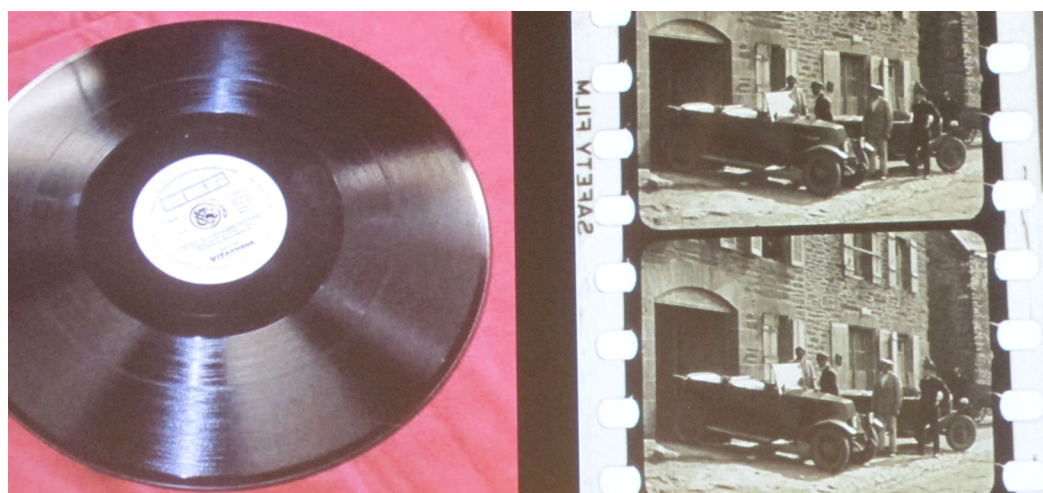
Fig. 28 and 29: Vitaphone film image and sound carriers (35 mm film, sixteen-inch electrical disc)
