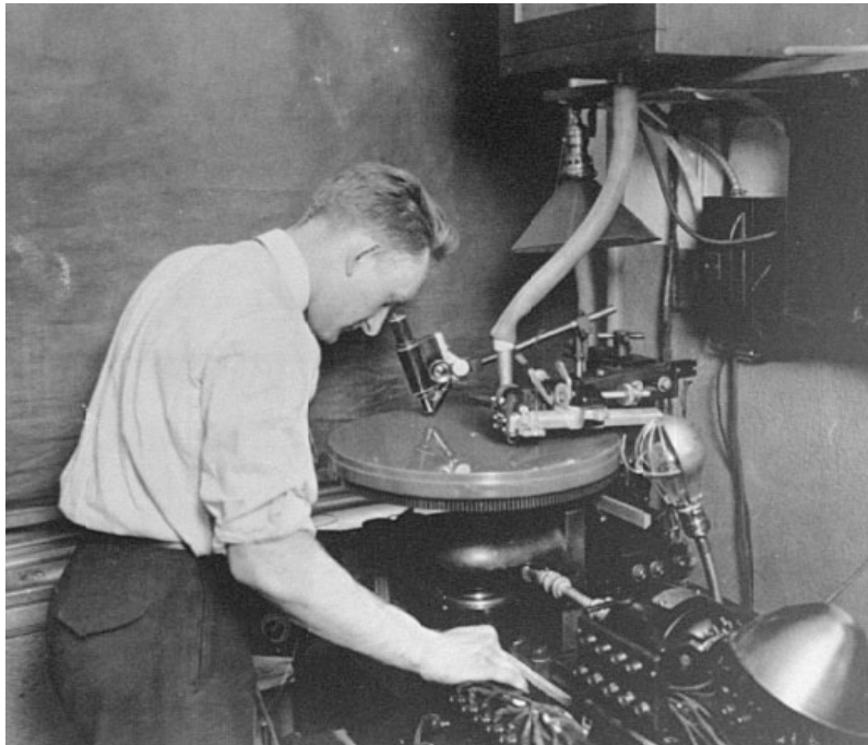
Fig. 30: Vitaphone engineer George Groves at a 1925 electrical disc-cutting lathe for sound movies [The Granger Collection, NYC]
