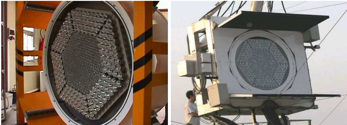
Figure 2.3: First MAGIC I camera. On the left: inside view of the hexagonal camera with the smaller pixels in the inner region surrounded by the bigger ones [42]. On the right: the camera installed on the telescope [41].
