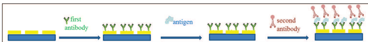
Figure 3.4 – Schematic representation of a sandwich assay amplified detection of protein. First, a layer of thiolated antibody is formed on the surface of gold pillars; after the antigen detection, the system is incubated with a second antibody.
