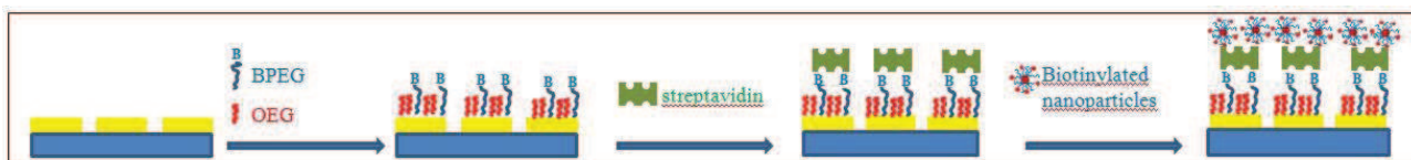
Figure 3.7 – Schematic representation the biotin-streptavidin sandwich assay: mixed SAM exposing biotin and -OH group is incubated with streptavidin, on which biotinylated nanoparticles are then linked.
