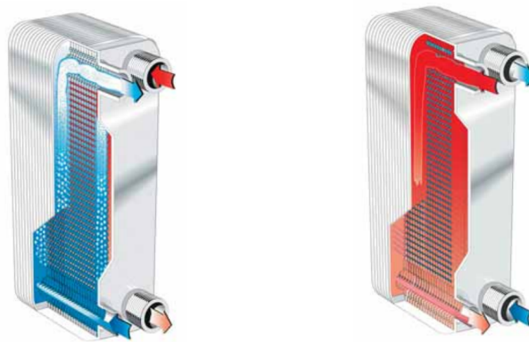
Figure 5.9: Plate heat exchangers in DX expansion and condenser configurations [?]
