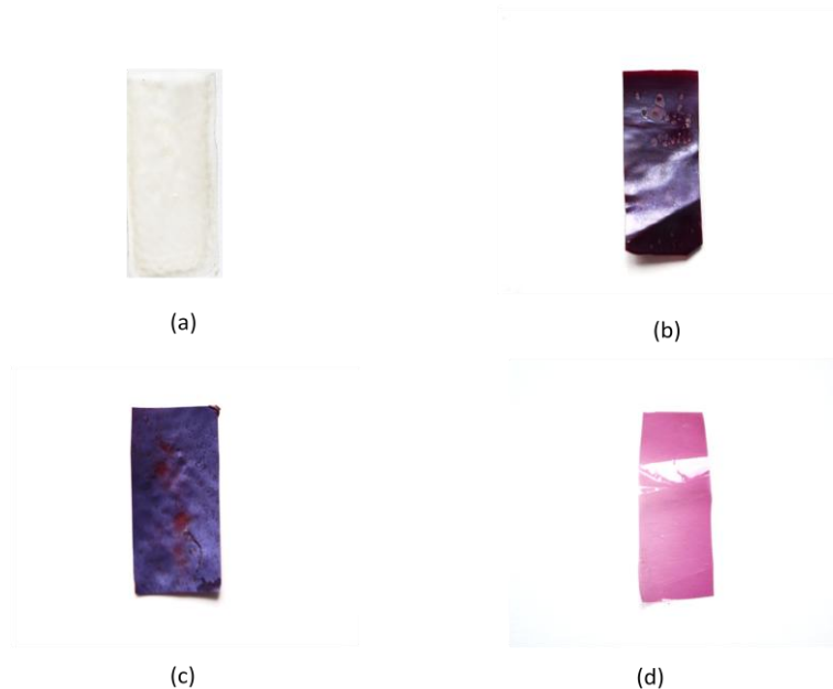
Figure 4.1 Photographic images (a) PVC with 20 \mu\text{l} OA (b) 5% TPP-PVC with 20 \mu\text{l} OA (c) 5% TPP-PVC with 40 \mu\text{l} OA (d) 1% TPP-PVC with 20 \mu\text{l} OA
