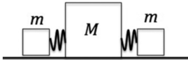
Figure V.2a. The mechanical system used in Dib's TE (2013): two blocks of mass m connected by two compressed spring to a central greater block of mass M . This is the initial configuration in the rest frame.
