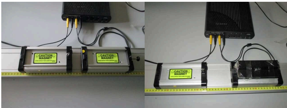
Figure VI.2. The colliding carts may be uncharged (empty, on the left) or one may be charged with up to three metal bars (on the right).
