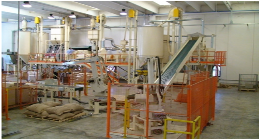
Fig 2 - Raw coffee cleaning machines before storage. Plants to automatize the receiving of raw materials that can reach the production facility in different modes or containers, such as:
