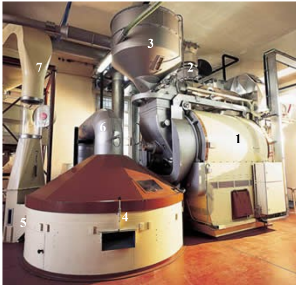
Fig 5 – Roaster machine: Tecnology of coffee, tea and other beverages (Source: Antoniazzi, 2008)
