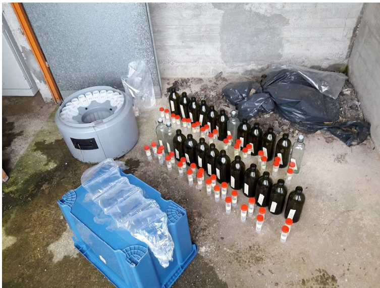
Figure 3.8: (a) The end-of-pipe manhole and the automatic sampler Sigma SD900 ready to take samples during storm events (the location is the same of the flow meter) and (b) bottles and tubes ready to divide samples for the laboratory analysis
