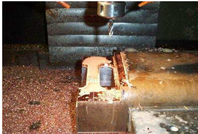
Figure 3.25: Manufacturing operation to obtain the tensile-test specimens [61].
