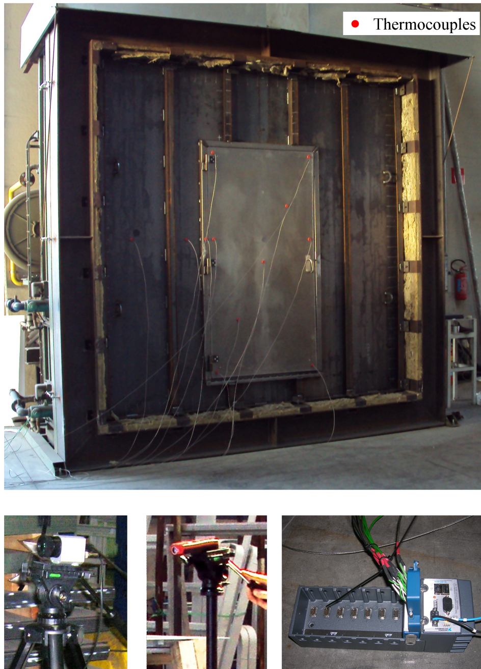
Figure 4.2: Experimental set up: thermocouples, thermographic camera, laser sensor and real-time controller.
