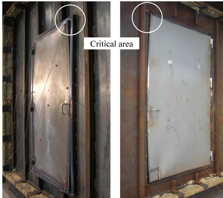
Figure 4.6: Typical deformed shape of fire doors during the test.
