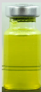
Figure IV. Visual aspect of transparent microemulsion containing 20% (w/w) oil with 3:1 ratio (lemon:peanut oil) added with 0.06% (w/w) curcumin, and an aqueous phase of 30% (w/w) Tween 80 in 0.8 M NaCl.
