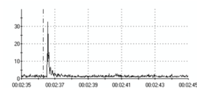
Figure 5.4: Filtered EMG signal showing an EBSR to a stimulus presented in correspondence to the dot-dashed vertical line.
