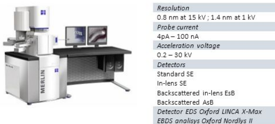
Figure 2.7. Image of the SEM instrument and its main specifications. 13
