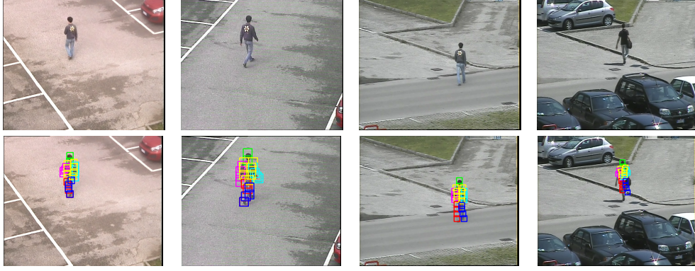
Figure 4.2: Examples of the computed body pose estimation using [150]. Top row shows four query images. Bottom row shows the corresponding detections and the estimated body parts. Lower limbs are depicted using red and blue while upper limbs are shown using cyan and magenta. The torso is shown in yellow and the head in green. The first three column show good results while the fourth column shows a good detection but a wrong pose estimation of the person body parts. Notice that in all four cases a perfect detection is achieved, and shadows and other objects in the scene do not affect the results.
