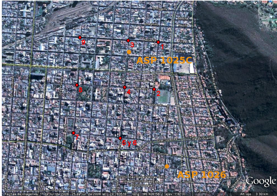
Figure 3.6: Red dots show the measurement points where the three-component seismometer Mark L4 - 1sec has been placed to acquire the environmental tremor. Each number correspond to the seismic station number in the following presentation of the SOM results. Yellow dots show the position of a pair of the available drillings (see fig. 3.7).
