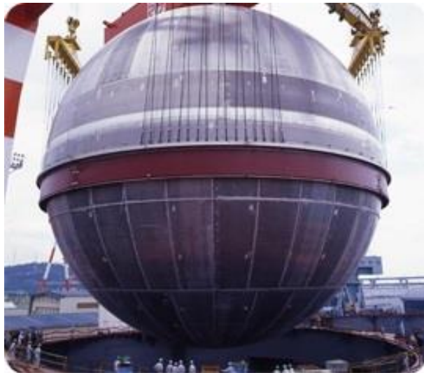
Figure 17. Typical prismatic and spherical B type tank [44, 45].
