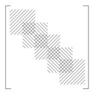
Figure 3.4: Matrix assembling for multi-element discretization
