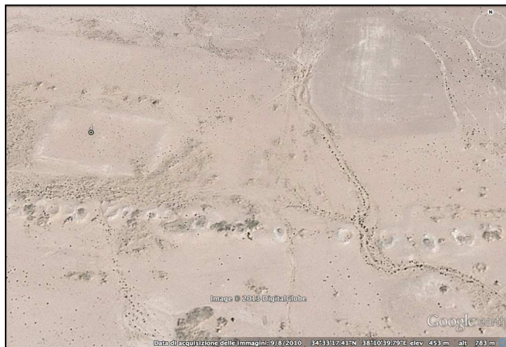
Fig. 4.18. The characteristic regular qanat 's holes on the ground. (Image produced from Google Earth)
