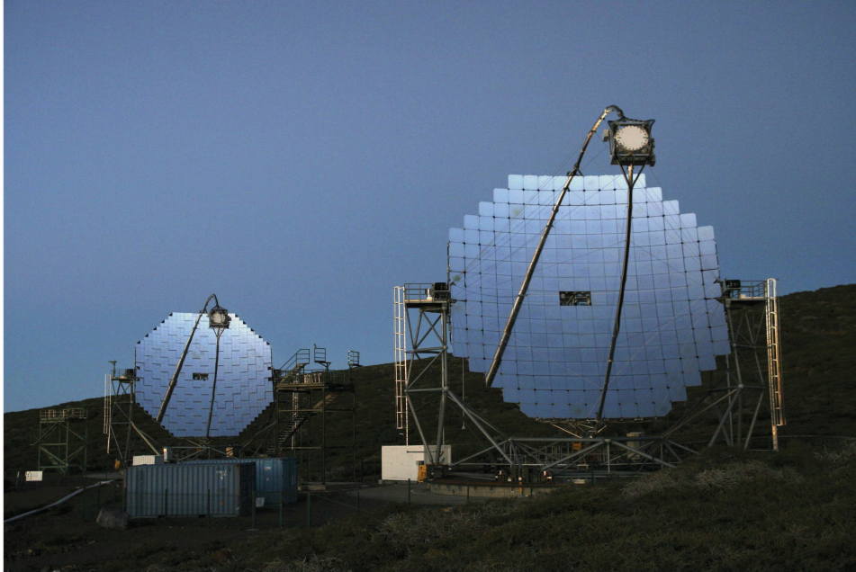
Figure 1.17: The two 17 m diameter MAGIC telescope system operating at the Roque de los Muchachos observatory in La Palma [33].
