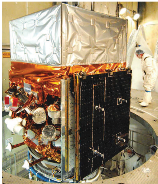
Figure 1.1: The Fermi spacecraft shortly before launch: the solar panels are folded at the sides, the GBM detector modules and the telemetry antennas can be seen on the left side, the LAT on the top. Picture taken from [1].
