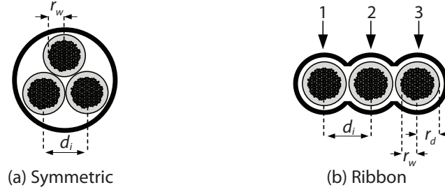
Figure 7.4: Cross sections of the two considered cables.
