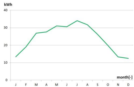
Figure 5.9 - Monthly production of a 1m 2 PV panel
