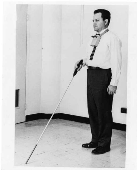
Figure 5.2: The Pathsounder - It is a mobility aid to assist the blind user to detect obstacles which his/her cane cannot reach. Source: http://webmuseum.mit.edu
