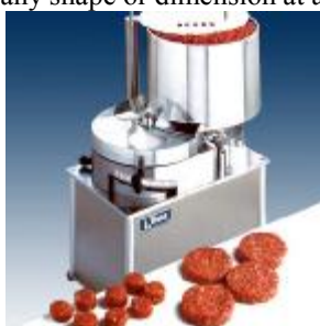
Figure 5.1 The MS-automatic moulding machine for hamburgers (Nilma, 2012).
