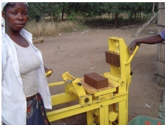
Fig. 4.12. Maputo (Mozambique), the preparation of the CEB
