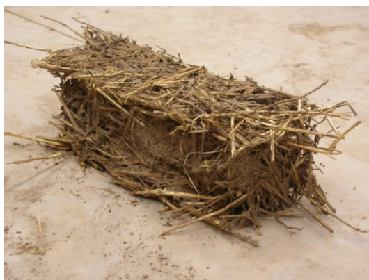
Fig. 4.7. Straw-loam after the drying process
