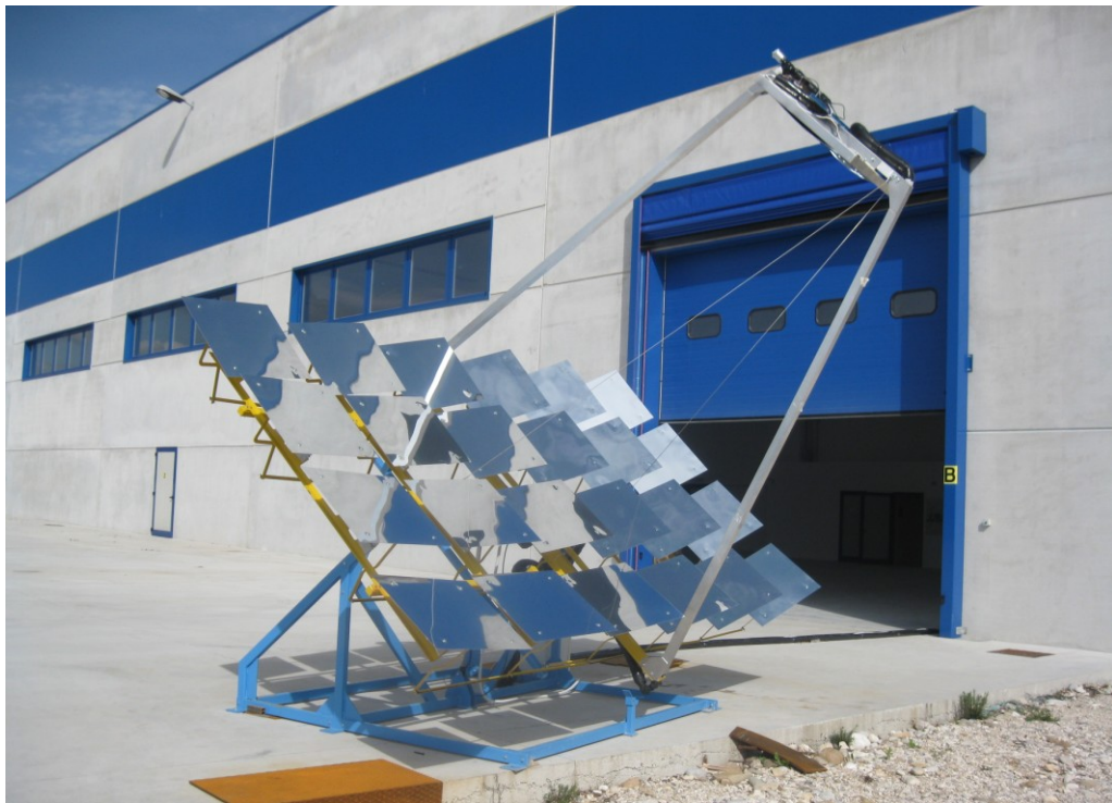
Fig.5. The prototype of the “Linear Mirror” The system consists of an array of plane mirrors, driven by only two motors
