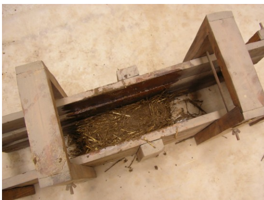
Fig. 4.6. Straw-loam in a formwork
