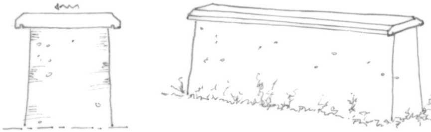
Fig. 5.89. Protecting the top of the walls with caps
