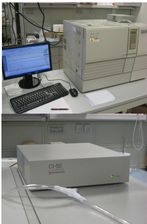
Figure 41: equipment used for MP analysis during the first part method development: GCxMS and CI-50 gas controller
