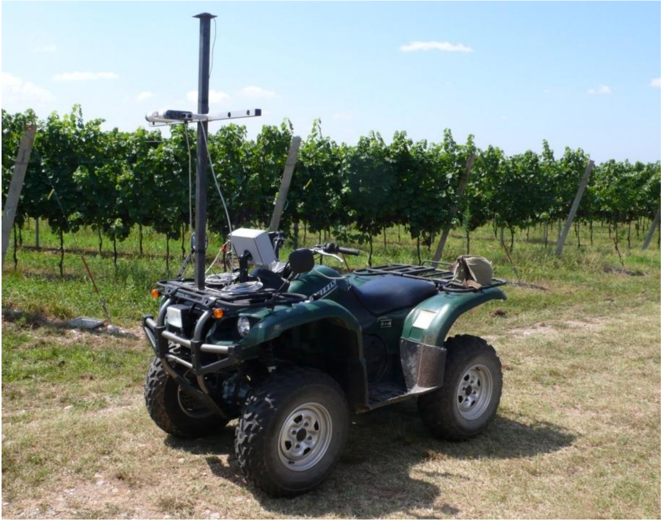
Figure 16: QUAD equipped with NDVI sensors and PC-datalogger;
