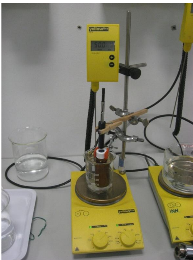
Figure 39: heated bath with brown vial and inserted fiber for SPME extraction
