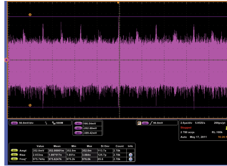
(b) The 3.3V power line in AC mode
