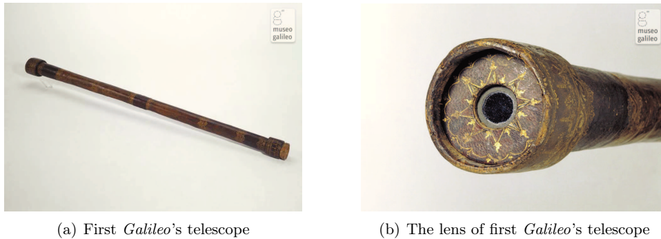
Figure 1.5: The first telescope built by Galileo Galilei (1609). The main tube is composed of wood lathes, covered by red-brown skin and gold friezes. The convex lens diameter is 37 mm and its focal length is 980 mm, while the eyepiece diameter is 22 mm with a focal length of -47,5 mm (a negative focal length means it is divergent). The telescope can magnify the objects by a factor of 21 times with a field of view of 15'. (Courtesy of Museo Galileo Firenze - photo Franca Principe)
