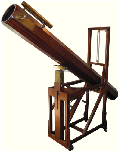
Figure 1.6: Model of telescope, exhibited in the William Herschel museum in Bath, which he discovered Uranus with. The power and magnification of his telescope was the secret of his success. It is 7 foot long and 6 inch diameter. Both mirrors, the main at the bottom of the tube and the secondary mirror near the top, were made of speculum metal.
