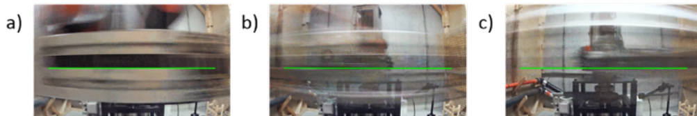
FIGURE 3.20: Qualitative estimation of the displacement of the rotating structure at different rotating conditions: 5 rpm (a), 100 rpm(b) and 250 rpm (c).
