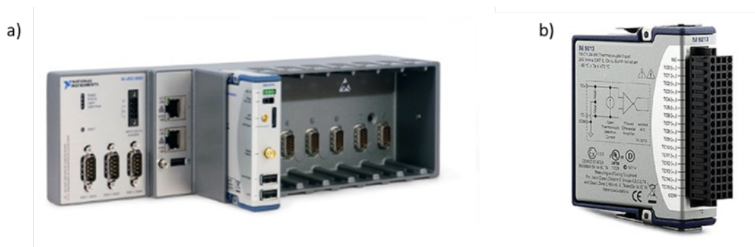
FIGURE 3.7: NI cRIO (a), NI 9213 module (b).
