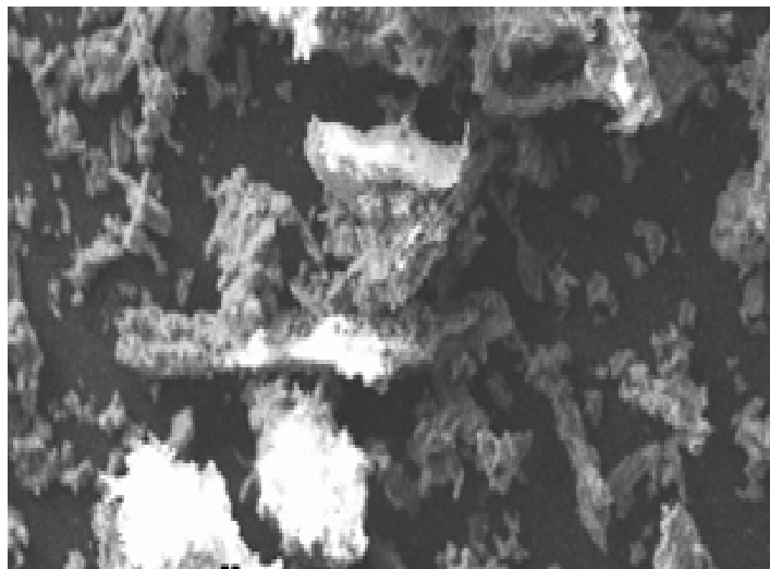
Figure 6.7: SEM photograph of the wood pellets at pyrolysis temperature of 400°C.
