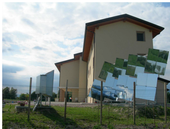
Figure 3.14: The Linear Mirror II, with the absorber.
