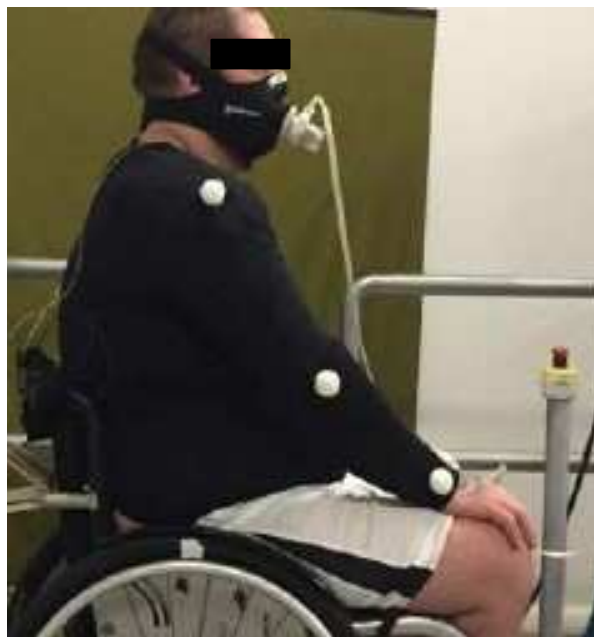
Figure 2.3. Markers positioning for kinematic analysis.
