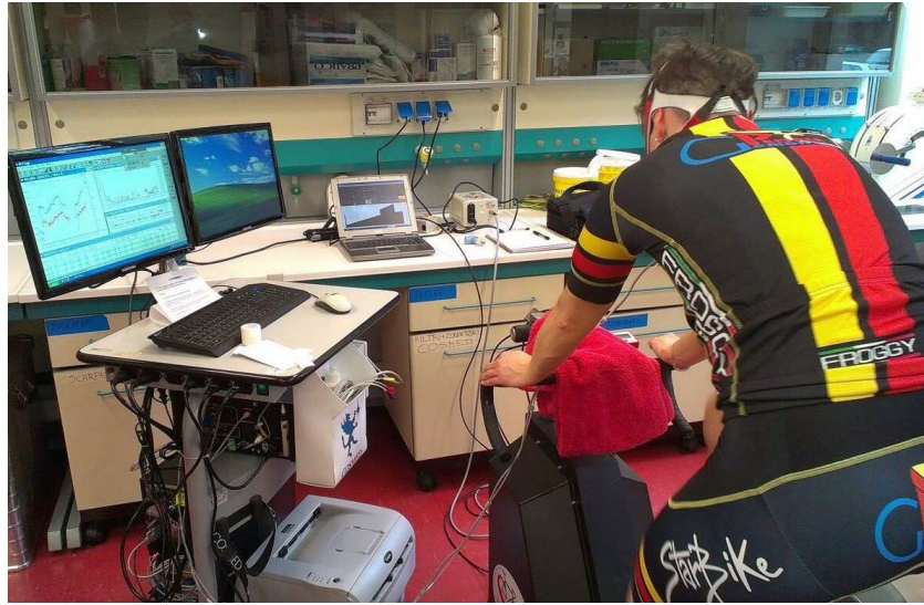
Figure 1.11. Metabolic cart for CPET connected to the mask during an incremental test at the cycle ergometer.
