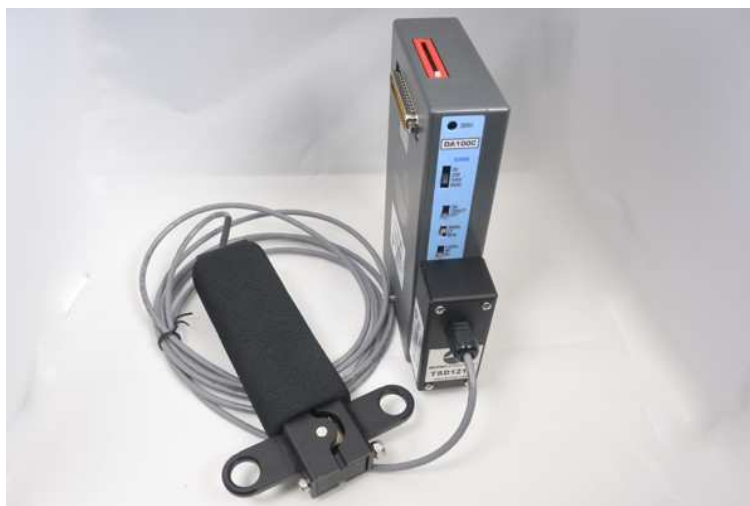
Figure 3.8. The TSD121C isometric dynamometer (Biopac Systems Inc., Santa Barbara, CA, USA). By www.biopac.com
