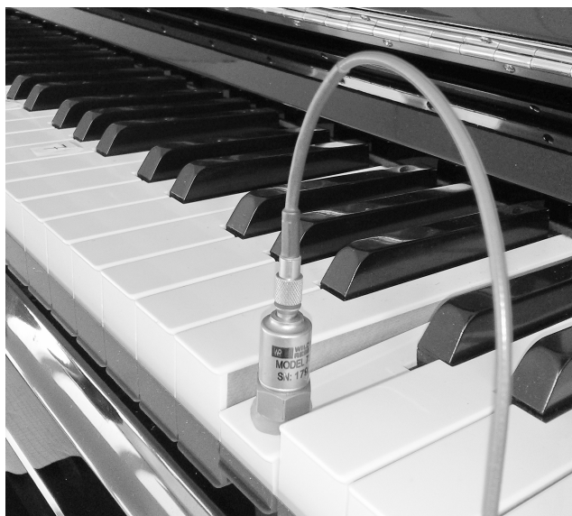
Figure 2: The vibration recording setup: A Wilcoxon Research 736 accelerometer is attached with adhesive tape to a key that is being played remotely via MIDI control
