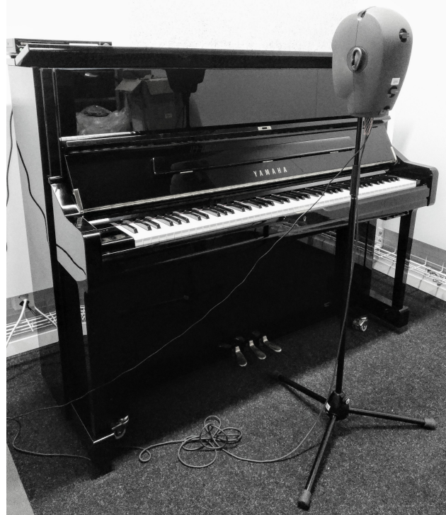
Figure 1: The binaural recording setup used in Zurich. The piano lid is in ‘semi-open’ position
