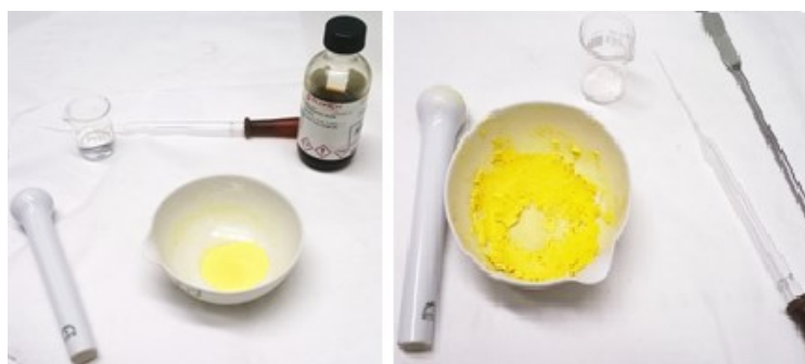
Figure 2.1: impregnation of Ce_{0.75}Zr_{0.25}O_2 mixed oxide
