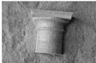
Figure 16 RP techniques with nylon powder for the Doric Capital
