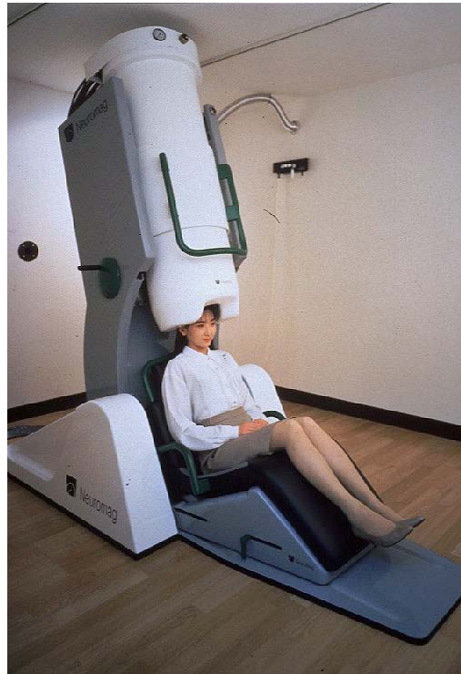
Figure 2.2: Apparatus for MEG, placed inside a magnetically shielded room. Source: Functional Neuroimaging ( http://www.psych.nyu.edu/pylkkanen/Neural_Bases/07_slides/05_Methods.pdf )[4]
