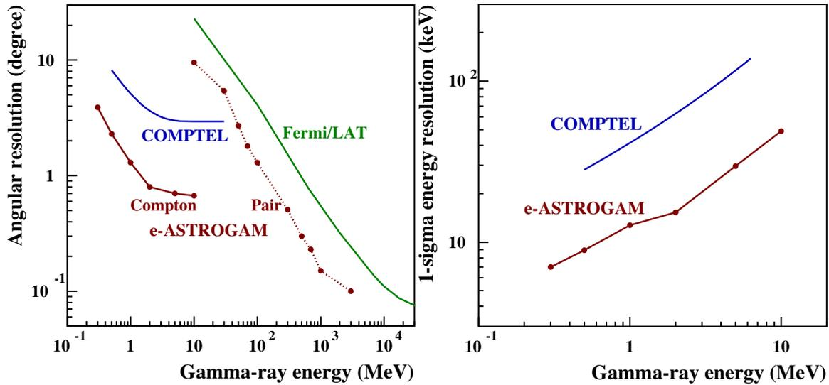
**Figure 3.** *Left panel* – e-ASTROGAM on-axis angular resolution compared to that of COMPTEL and *Fermi/LAT*. *Right panel* –  $1\sigma$  energy resolution of COMPTEL and e-ASTROGAM in the Compton domain. From [1].
