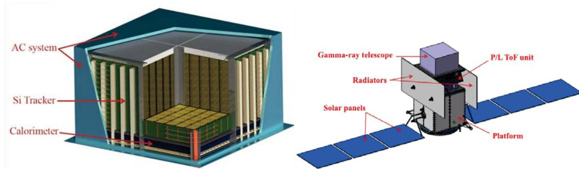
**Figure 2.** *Left panel* – overview of the scientific instrument. *Right panel* – the scientific instrument on top of the platform. From [1].
